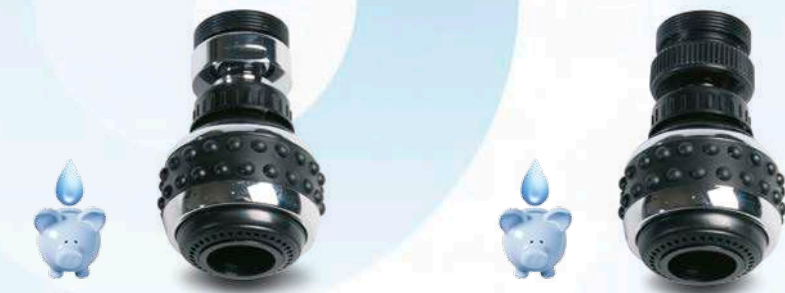
ATOMIZADOR CON RÓTULA METALICA Y ECONOMIZADOR Posiciones chorro y ducha. Rosca H-22 x 100 y M-24 x 100 indistintamente. Latón y ABS cromados. ATOMIZER WITH METALLIC BALL FITTING AND ECONOMISER Jet and shower position. For F-22 x 100 and M-24 x 100 screw thread. In chromium-plated brass and ABS.
